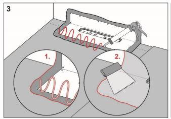
Apply Zebra barrier adhesive on the drain collar and Weber foil and joint adhesive or Zebra Tätmembran to the rest of the floor and wall area.
