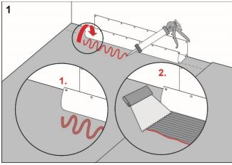
Apply Zebra barrier adhesive to the floor and wall areas which the drain collar will cover. Spread the adhesive with a fine-toothed adhesive spreader.
