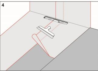
Install Zebra Duk and overlap the drain collar by a minimum of 35 mm. Seal all seams with Zebra Tätmembran.
