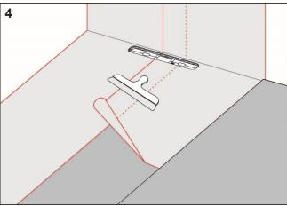
Install the foil and overlap the drain collar by a minimum of 50 mm. Seal all seams with 2K foil and joint adhesive or membrane and foil glue.
