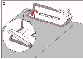
Unfold the collar on the floor and wall. Press the collar firmly into place and ensure that no wrinkles or blisters occur.
