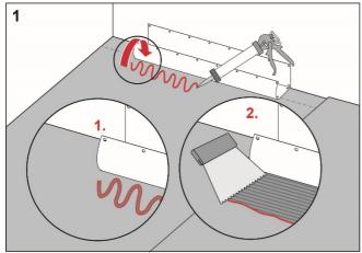
Apply accessory adhesive or 2K foil and joint adhesive to the floor and wall areas which the drain collar will cover. Spread the adhesive with a fine-toothed adhesive spreader.
