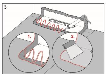
Apply 2K foil and joint adhesive or accessory adhesive at least 50 mm on the drain collar. Apply membrane and foil adhesive or 2K foil and joint adhesive to the rest of the floor and wall area.
