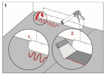
Apply Sopro Rocofix 818 mounting adhesive to the floor and wall areas which the drain collar will cover. Spread the adhesive with a finetoothed adhesive spreader.
