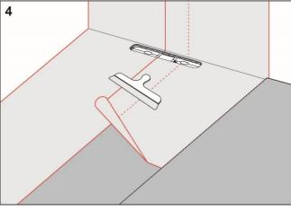
Install Sopro Folie and overlap the drain collar by a minimum of 50 mm. Seal all seams with Sopro FDK 415 fixing adhesive and sealant.
