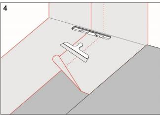
Install Schönox Folie and overlap the drain collar by a minimum of 50 mm. Seal all seams with Schönox iFIX or Schönox HA.
