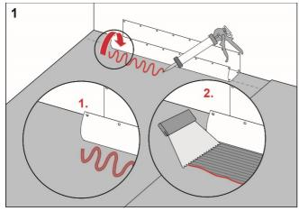
Apply Wetstop Foilseal to the floor and wall areas which the drain collar will cover. Spread the adhesive with a fine-toothed adhesive spreader.
