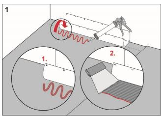
Apply Midun Skarvlim Våtrum to the floor and wall areas which the drain collar will cover. Spread the adhesive with a fine-toothed adhesive spreader.
