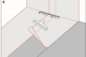
Install Midun Våtrumsfolie and overlap the drain collar by a minimum of 35 mm. Seal all seams with Midun Tätmembran.
