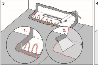
Apply Midun Skarvlim Våtrum on the drain collar and Midun Tätmembran to the rest of the floor and wall area.
