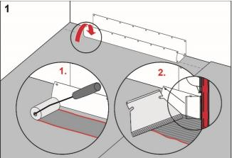
Apply Mapei Mapeguard WP Adhesive on the floor and wall areas which the drain collar will cover. Spread the adhesive with a brush, roller or adhesive spreader.
