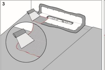
Apply Mapei Mapeguard WP Adhesive on the drain collar and on the rest of the floor and wall area.
