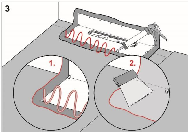
Apply LIP Skarvlim MSP or LIP 2K Folie W-Lim on the drain collar and LIP 2K Folielim W-Lim to the rest of the floor and wall area.
