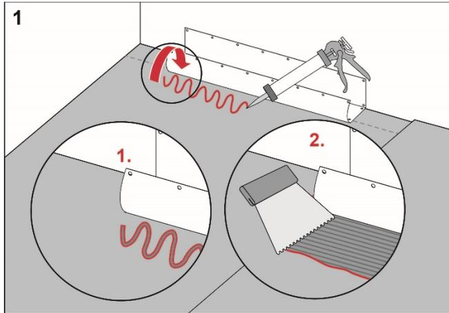
Apply LIP Skarvlim MSP to the floor and wall areas which the drain collar will cover. Spread the adhesive with a fine-toothed adhesive spreader.
