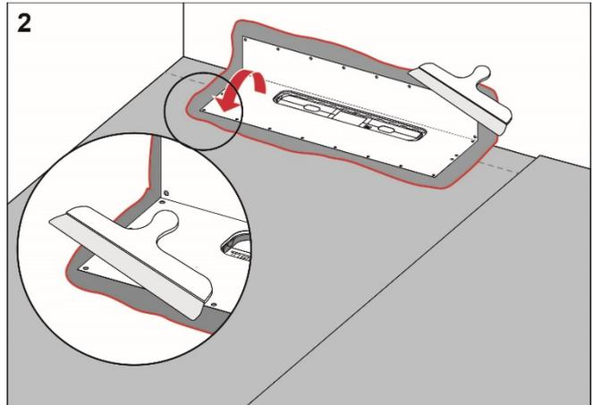
Unfold the collar on the floor and wall. Carefully smooth out the collar and ensure that no wrinkles or blisters occur.
