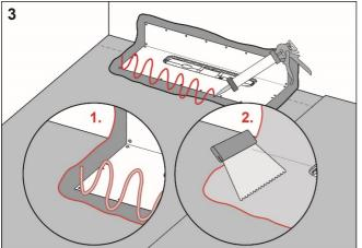
Apply Kiilto Keraseal on the drain collar and Kiilto K2 or Kiilto M1000Eco to the rest of the floor and wall area.
