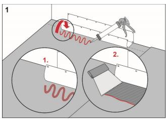
Apply Kiilto K2 or M1000eco to the floor and wall areas which the drain collar will cover. Spread the adhesive with a fine-toothed adhesive spreader.
