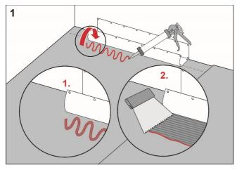
Apply Kerakoll Aquastop Nanosil to the floor and wall areas which the drain collar will cover. Spread the adhesive with a fine-toothed adhesive spreader.
