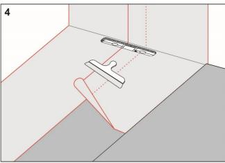
Install Kerakoll Folie and overlap the drain collar by a minimum of 50 mm. Seal all seams with Kerakoll Nanodefense Eco.
