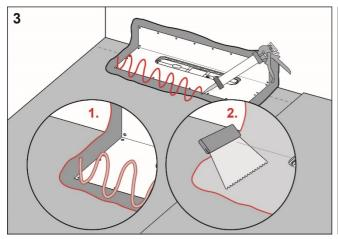
Apply GKHero Pro Folielim on the drain collar and GKHero Pro Våtrumsmembran to the rest of the floor and wall area.
