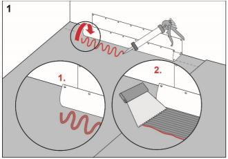
Apply GKHero Pro Folielim to the floor and wall areas which the drain collar will cover. Spread the adhesive with a fine-toothed adhesive spreader.
