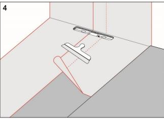
Install GKHero Pro Våtrumsfolie and overlap the drain collar by a minimum of 35 mm. Seal all seams with GKHero Pro Våtrumsmembran.
