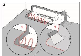
Apply Ecodur Folielim on the drain collar and Ecodur Tätmembran to the rest of the floor and wall area.
