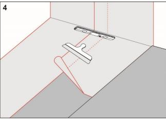
Install Ecodur Tätfolie and overlap the drain collar by a minimum of 35 mm. Seal all seams with Ecodur Tätmembran.
