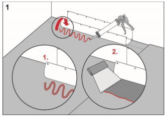
Apply Ecodur Folielim to the floor and wall areas which the drain collar will cover. Spread the adhesive with a fine-toothed adhesive spreader.
