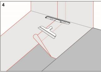
Install Centro TM#Folie and overlap the drain collar by a minimum of 35 mm. Seal all seams with Centro TM#Tätmembran.
