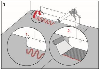
Apply Centro TM#Folielim to the floor and wall areas which the drain collar will cover. Spread the adhesive with a fine-toothed adhesive spreader.
