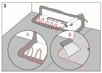
Apply Centro TM#Folielim on the drain collar and Centro TM#Tätmembran to the rest of the floor and wall area.
