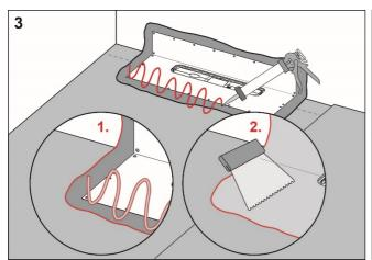
Apply CC Höganäs FB44 Tublim to the drain collar and CC Höganäs FB7 Folielim to the rest of the floor and wall area.
