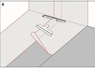
Install CC Höganäs Folie and overlap the drain collar by a minimum of 50 mm. Seal all seams with CC Höganäs FB7 Folielim.
