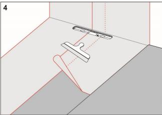
Install Bostik Folie Universal and overlap the drain collar by a minimum of 50 mm. Seal all seams with Bostik Membran Universal or Bostik Foil Adhesive Universal.
