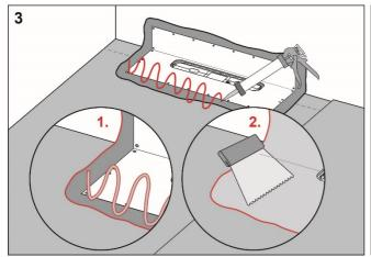
Apply Bostik Foil Seal Grab on the drain collar and Bostik Membran, Foil Tac 1C or Foil Seal Cement on the rest of the floor and wall area.
