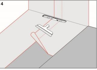
Install Alfix Våtrumsmatta Pro and overlap the drain collar by a minimum of 50 mm. Seal all seams with Alfix 2K Tätningsmassa.
