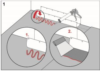
Apply Alfix 2K Tätningsmassa to the floor and wall areas which the drain collar will cover. Spread the adhesive with a fine-toothed adhesive spreader.
