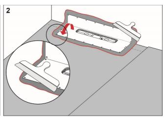
Unfold the collar on the floor and wall. Carefully smooth out the collar and ensure that no wrinkles or blisters occur.
