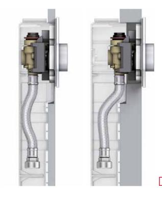
Traditional RTL boxes can protrude a long way into the room depending on the construction of the wall. TECE has solved the problem by developing a mounting plate with a special depth adjustment system, which always provides a consistent appearance - in all rooms, on every wall.
